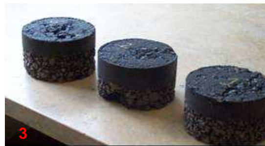
3. Samples after soaking in fuel
