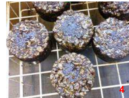
3. Samples after soaking in fuel
