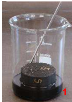
1. Test samples parcialy soaked in fuel
