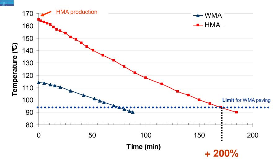
A HMA with chemical additives may be paved after a hauling time ~3 times longer
